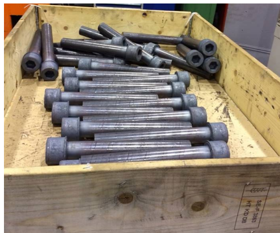
Figure 15 – Pameto manufactures M42 bolts in M-Steel.
