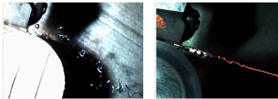
Figure 5 – Using M-Steel in hard part turning can result in chips glowing with heat as shown in the photograph on the right.
